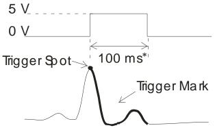
\*The model 3000T that is available in Japan may be set to generate a trigger pulse of 50ms (width) and 0-5V (amplitude) instead of the standard trigger pulse of 100ms and 0-5V.
